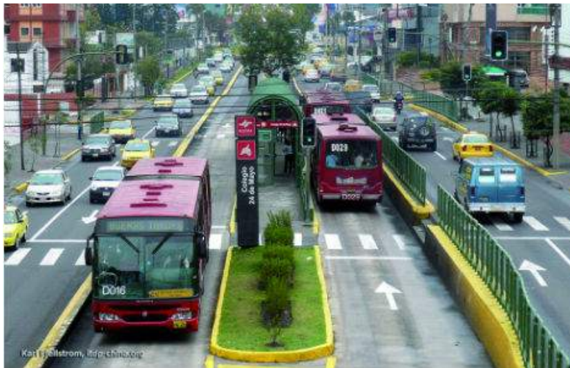
Figure 11: Example of a ground level BRT stop & bus lanes on the BRT system in Bogota, Colombia
